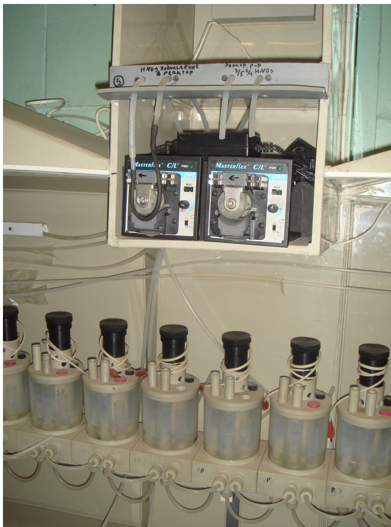
Figure 24 - Cascade equipment for the separation of individual REE (Romedmet, RF)
