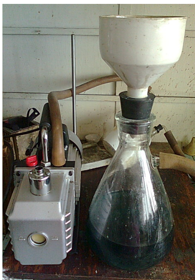
Figure 2 - Vanadium-containing solution, after leaching
