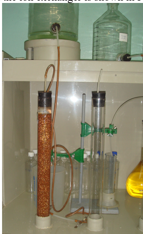
Figure 22 - Sorption extraction of the amount of REE from technological solutions
